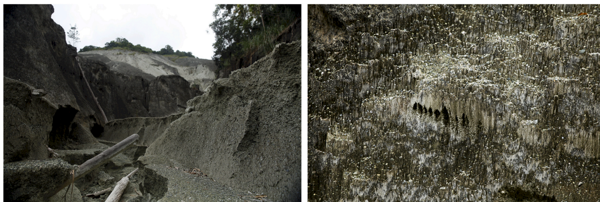
Fig. 14. Eroded asbestos tailings south of Bulembu. Right image is detail, showing the cm high earth pyramids with asbestos fibre that will be eroded by rainfall events (width \approx 1 m).
